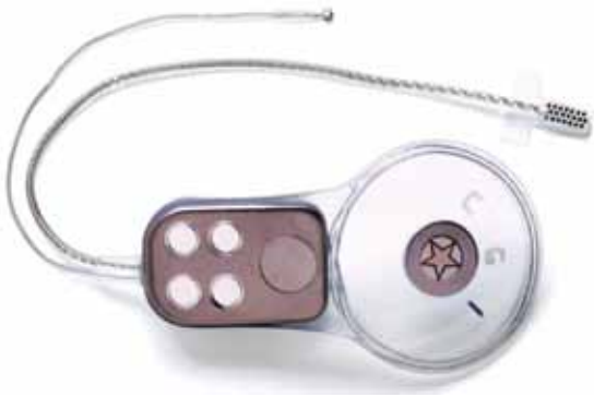
Figure 4: Multichannel auditory brainstem implant. Image courtesy of Cochlear™ Americas, © 2009, Cochlear Americas
